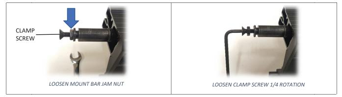
ISSUE: WHEN ASSEMBLING FRONT END, THE RISER AND MAINFRAME ARE NOT TIGHT TOGETHER.
