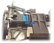
MIN. GAP BETWEEN RISER & MAINFRAME
