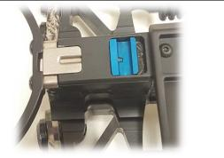
RELEASE SWITCH IN CLOSED POSITION
