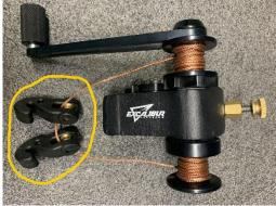
**Before you begin:** Remove the C2 crank from the crossbow by loosening the brass thumb screw and pulling the crank off the crossbow stock.
