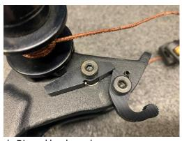
**Step 2:** Cut the rope and remove the hooks and rope from the crank. Discard hooks and rope.
