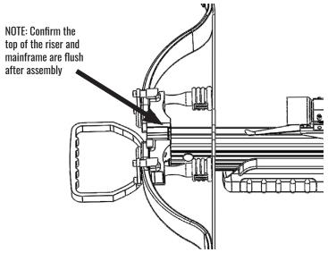
**Step 2**: Insert barrel nut into hole in mainframe, ensure one of the threaded holes in the barrel nut is oriented towards the front of the bow, equal amounts of the barrel nut should protrude from both sides of mainframe once properly centred:
