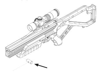
Step 4: Insert 5/16-18 x 2.25" flat head cap screw through the riser assembly and thread into the barrel nut, you may need to rotate the barrel nut slightly to perfect the thread and fastener alignment. Tighten with 3/16" allen key:
