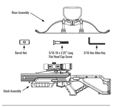
Step 3: Align the riser assembly with the stock assembly:
