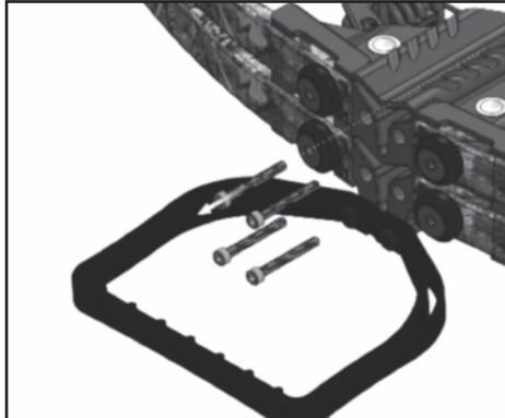
**4. Install previously removed screws and torque to 22 in-lb.**
