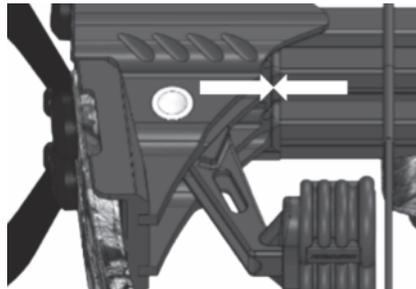
**There should be no gap between riser and mainframe visible.**
