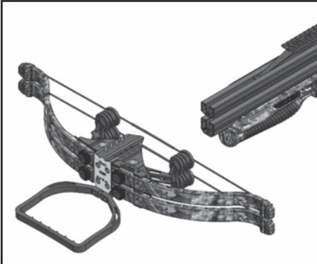
**3. Install limb assembly to front of mainframe**
