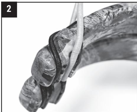
2. The stringing aid should be pulled toward the trigger unit with the serving beneath the upper hold down spring [FIG 3]. Proceed to the Unstringing/Adjusting brace height section.
