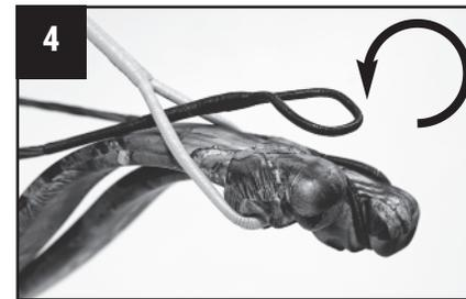
4. Install the charger EXT crank handle and follow decocking instruction to let the DualFire Stringing Aid down until no draw weight is felt on the crank handle, verify the brace height using the markings on the mainframe. If more twists are required repeat steps 1-3. If the brace height is correct, detach cocking aid hooks and stow.
