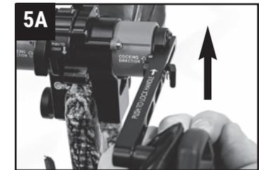
6. Once you have confirmed that the trigger catch has captured the crossbow string. Immediately place the safety into the "SAFE" by moving it into the up position.
