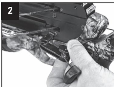
**NOTE: The DualFire Decocking Adapter hook attaches to the crank rope via the brass pulley.**
