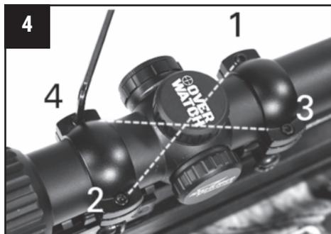
**Note: Look through the scope periodically during step 4 to verify the reticle remains level with the integrated stock level.**
