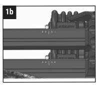
1. Place your foot firmly in the stirrup, lift the DualFire Stringing Aid (positioned in the previous instruction on page 22) with the Charger EXT (refer to cocking instructions on Page 10) until the bow string has sufficient slack to be removed from one limb tip, an extra turn or two of the crank handle will create the required additional slack to account for the shortened/twisted up string in the next step(s) [FIG 2]
