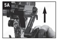
6. Once you have confirmed that the trigger catch has captured the crossbow string. Immediately place the safety into the "SAFE" by moving it into the up position.
