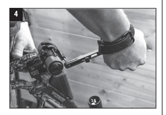
Apply slight pressure to the REAR (lower deck) trigger while rotating the crank handle clockwise with increasing pressure. Once the trigger activates, full draw weight will be transferred to the crank.
