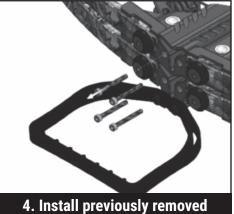
4. Install previously removed screws and torque to 22 in-lb.
