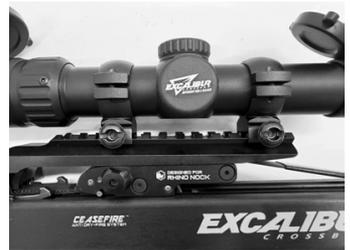
**STEP 2B:** With a screwdriver, tighten the large locking nuts at the side of the rings.
